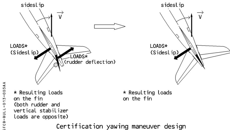
JAR/FAR 25 requires the above yawing maneuver to be analyzed over the full range of specified conditions. The most severe loads imposed on the vertical stabilizer and rudder are identified.
