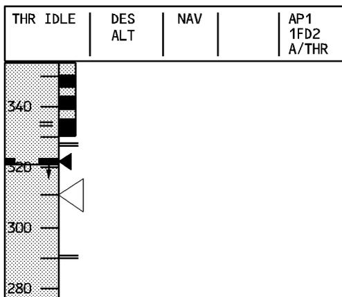
Consequently, when in managed descent and on idle segment, the flight guidance has 2 parameters to adjust in order to keep the aircraft on path : the IAS, which may vary within the speed target range and, the thrust which may vary between Idle and Idle + DELTA, while the ATHR is in thrust mode.
