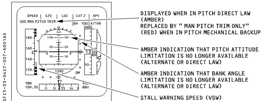
At low speed, the change in the speed scale is very noticeable. VLS remains, but  $V_{\alpha}$  PROT and  $V_{\alpha}$  MAX disappear, replaced by a single black and red strip, the top of which is stall warning speed. Unlike VLS, which is stable, VSW is g sensitive so as to give additional margin in turns. As mentioned above, ALTERNATE reverts to DIRECT law for landing at 100 feet.
