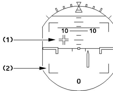
R The PFD includes a symbol (1) that is the sum of sidestick positions given to the computers. It permits the PNF to check that the PF is making an appropriate control input during takeoff roll.
