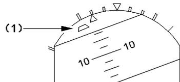
On the ground the aircraft is conventional. The pilot uses rudder to maintain direction. He should rotate to about 12.5° of pitch and adjust as required. The sideslip indication (1) changes to the engine-out mode (blue). When it is centered, the aircraft is close to the zero aileron position (best drag condition). It is therefore important to zero the slip indication accurately.
