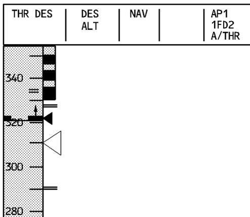
If the aircraft still tends to deviate above the path and the IAS gets close from the upper limit of the speed target range, the ATHR commands idle thrust so as to keep  $VDEV=0$ . THR IDLE is then displayed on the FMA.
