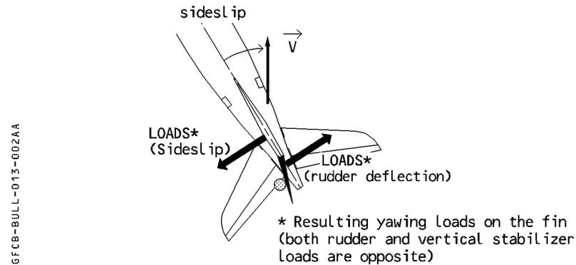
3 - With the airplane yawed to the steady-state (static) sideslip angle corresponding to the above rudder deflection, the certification regulations assume that the rudder pedal is released to neutral.
