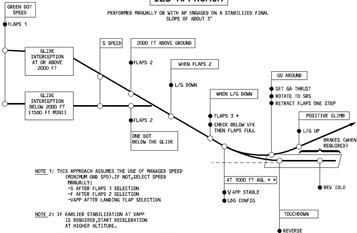
**NOTE 1:** THIS APPROACH ASSUMES THE USE OF MANAGED SPEED (MINIMUM GND SPD). IF NOT, SELECT SPEED MANUALLY:
