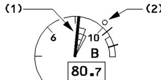
Thrust management is very easy. The pilot selects a FLX thrust by stopping the thrust levers in the FLX/MCT detent and checking that the resulting N1 (or EPR) (1) is compatible with N1 (or EPR) target (2). For maximum takeoff thrust, the pilot moves the thrust levers fully forward and makes the same thrust check (N1 or EPR).
