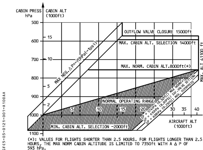
*Note* : Maximum differential pressure and safety valve setting tolerance = ± 7 hPa (0.1 psi)
