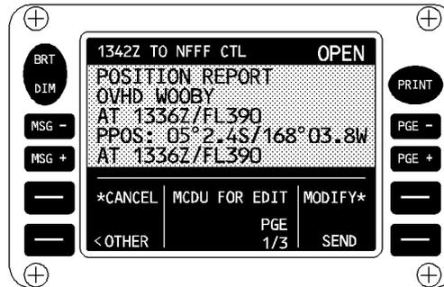
The pilot may modify it by using the MODIFY function key. Then, he sends it to the ATC. He may also use the MODIFY function key to update the parameters displayed on the DCDCU before sending the position report.
