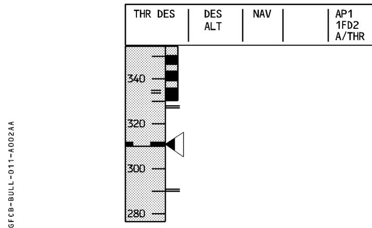
If for any reason the aircraft tends to deviate above the path, the IAS will increase with regards to the target within the speed target range so as to keep  $VDEV=0$ .
