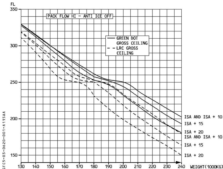
*Note : If severe icing conditions are encountered, ice formation may build up on non heated structure and therefore the ceiling will be reduced by 2500 feet.*
