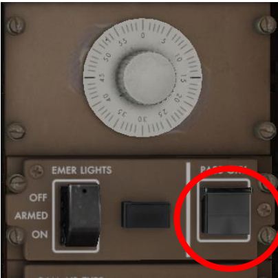
Emergency Lights Switch guarded and armed, PASS(engers) OXY(gen) Light should be OFF.
