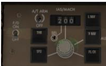
Mode Control Panel,
