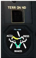
This panel concern the pressure for the brakes. This panel is locate in the Main Instrument Panel.
